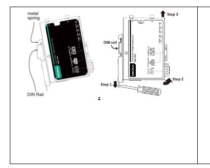
www.moxa.com No change in the installation method; . Insert the upper lip of the DIN-rail kit into the mounting rail, and press the AWK-1137C towards the mounting rail until it snaps into place. The new DIN-rail kit is provided with a slider that makes removing the AWK-1137C from a DIN rail a lot easier as shown in the following illustration: STEP 1: Pull down the slider on the 0 DIN-rail kit with a screwdriver. STEP 2 & 3: Slightly pull the 0 AWK-1137C forward and lift it up to
